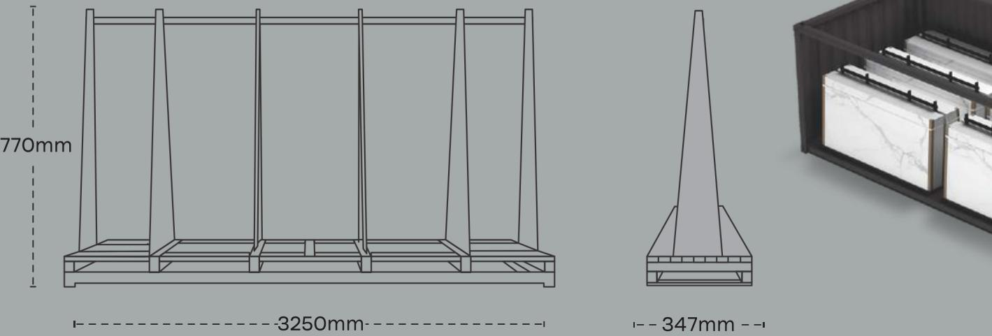
The A-frames should always be handled carefully, one at a time, to avoid instability or collapse. When moving the pallet, it must be secured with at least one vertical sling. Protective cardboard should be positioned at the height of the ratchet to prevent it from impacting or scratching the slab. When at rest, and if the goods are not strapped or secured with slings, vertical poles must be placed to stabilize the load in case of tipping.
